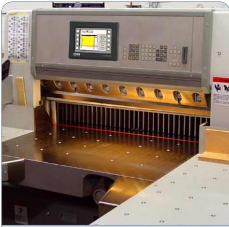
The intelligent capabilities of the QTERM-Z60 allows it to monitor and adjust the operation of an industrial shearing machine.
