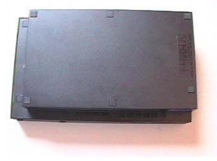
Remove all the screw covers. (There should be 6 screw covers, 4 made of rubber (outer edges) and 2 made of plastic (in the middle), that need to be removed. You can use a small flat blade screwdriver for this. There should be 2-4 more screw covers on the **outer** side of the base, underneath the controller ports. The older model PS2's have 4 screw covers, while the newer ones have only 2. Remove them all, and you should now have a total of 8-10 screws unveiled. Set the screw covers aside.
