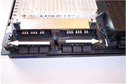
Once the console is flipped upside down just pull up on the case from the back. Be careful when removing the case so that it clears the USB connectors in the front. Once they are clear set aside the cover.
