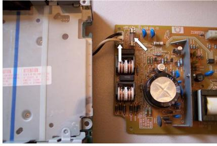
When you are done and ready to reassemble just reverse the procedure. Just be careful when plugging the power supply board back into the connector to make sure all the pins line up correctly.
