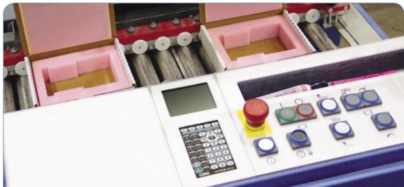
The components of the VTERM-G55 (module) were integrated into the panel of this packaging machine.
