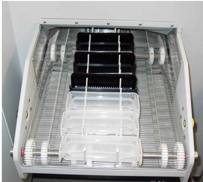
Complete cleaning and drying of plastic carriers in AAT's conveyORIZED and batch cleaning systems
