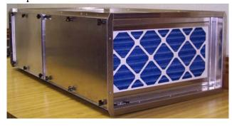
The unit is typically suspended above a drop ceiling and air from the contaminated space is ducted to it. The cleansed air is then either recirculated back to the space or exhausted from the area to create negative pressure.
