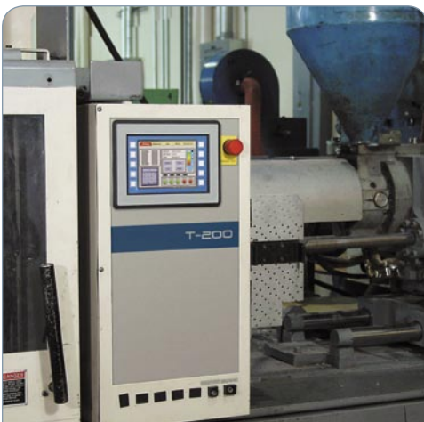
The intelligent capabilities of the QTERM-G70 allows it to monitor and adjust the hopper levels of an injection molding machine.
