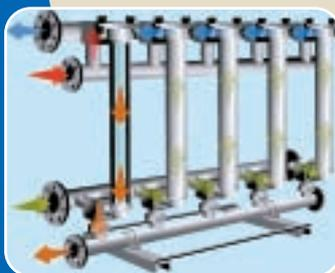
An external backwashing system utilizes an additional header at the top of the unit. This header introduces a separate cleaning liquid (typically water) to backwash the filter element to the drain.
