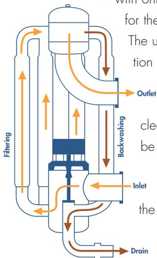
The unit features a configuration of up to 8 tubes surrounding a central cleaning valve. During backwash, a diverter inside the cleaning valve rotates to the tube to be cleaned. This closes the tube to the incoming process liquid and opens it to the atmosphere (via the drain line). The result causes outlet process liquid to flow in reverse through the element, cleaning it of contaminants and expelling them through the drain.
