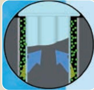
Process liquids flow into the housing at the inlet at its base and pass across the filter media from the outside inward. Because of this flow path, contaminants collect on the outside of the filter element slowly forming a cake, removing smaller particles.
