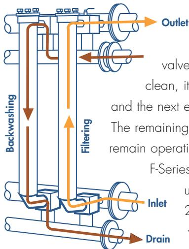
Our flagship tubular systems. During backwash, a single tube is taken off-line from the process flow via a three-way valve. Once an element is clean, it is returned to service and the next element may be cleaned. The remaining elements in the filter remain operational throughout this cycle.
