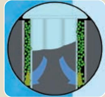
During backwash (triggered by time or pressure differential), a valve switches one station's flow from the inlet header to the drain header to facilitate reverse flow. Liquid is run in reverse through the system to remove contaminants from the media. Contaminants and cleaning fluid are expelled through the drain header at the base of the unit.
