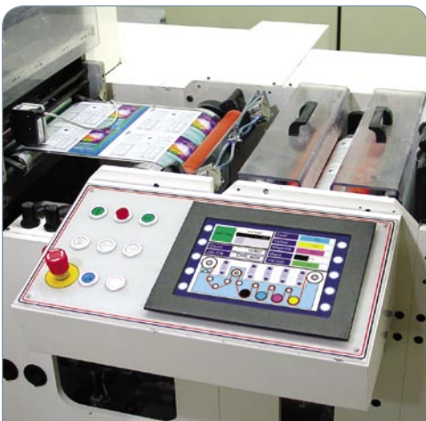
The QTERM-G75 serves as a control panel for a label printer.
