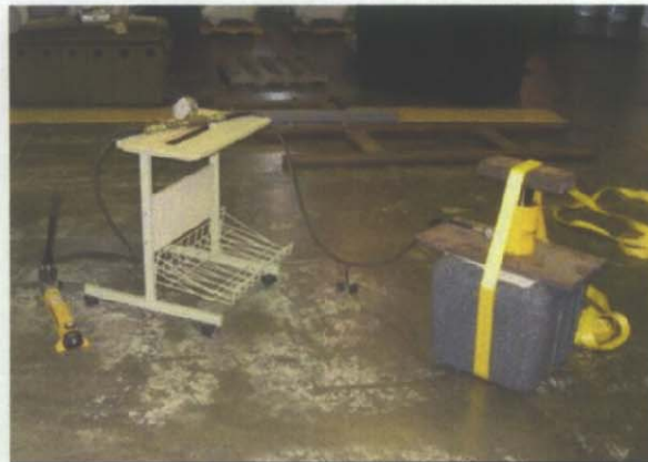
Photo 3: Frame Load Test on Eonian Urn Burial Vault
