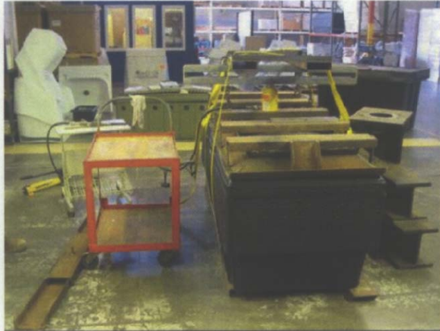
Photo 1: Frame Load Test on Endurance Burial Vault (Full size)
