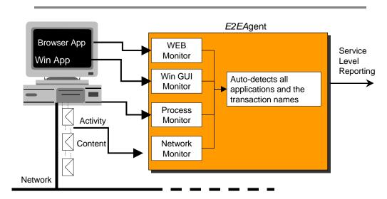
The agent employs multiple techniques to identify significant transaction start/stop markers while monitoring the request/response cycles. Each agent monitors several sources for significant events including:
