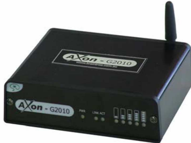
EFT to IP Gateway – answers the call from the pinpad and converts it to IP for carriage over a DSL network
