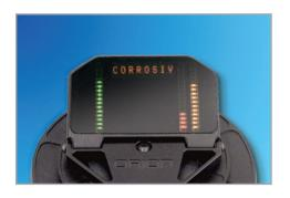
The GREEN LEDs indicate the transmit power level.
