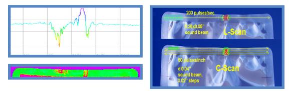
The high resolution Seal-Scan<sup>™</sup> takes 200-250 readings per second. The signal digitized and presented as 6000 shades of color. The space resolution is as small as 0.5mm. A single linear scan (L-Scan) takes only a few seconds and presents the quality of the seal as a line graph.
