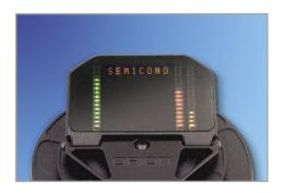
A strong RED response indicates electronics contained in potential contraband such as a cellular phone (the red LEDs represent the 2nd harmonic).
