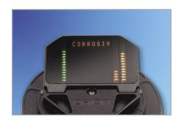
The GREEN LEDs indicate the transmit power level.
