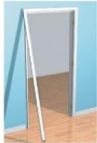
2. Use a reciprocating saw to cut nails where pieces will be installed.
