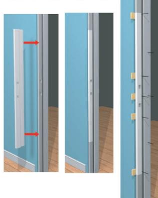
4. Use a reciprocating saw to cut nails where Hinge Shields will be installed.
