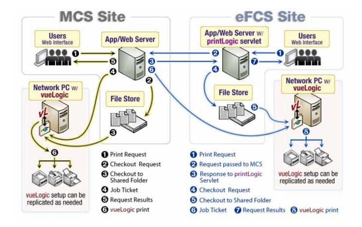
The diagram below shows the basic structure and process flow for **printLogic**:
