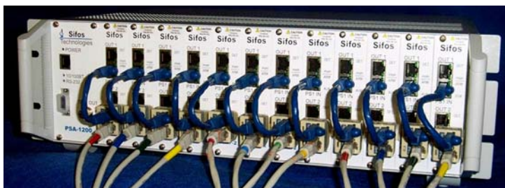
Figure 13: PSA with Port Combiners for Mid-Power PSE Testing.
