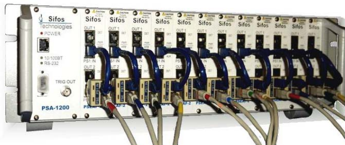
Figure 1. PSA Port Combiner Setup
