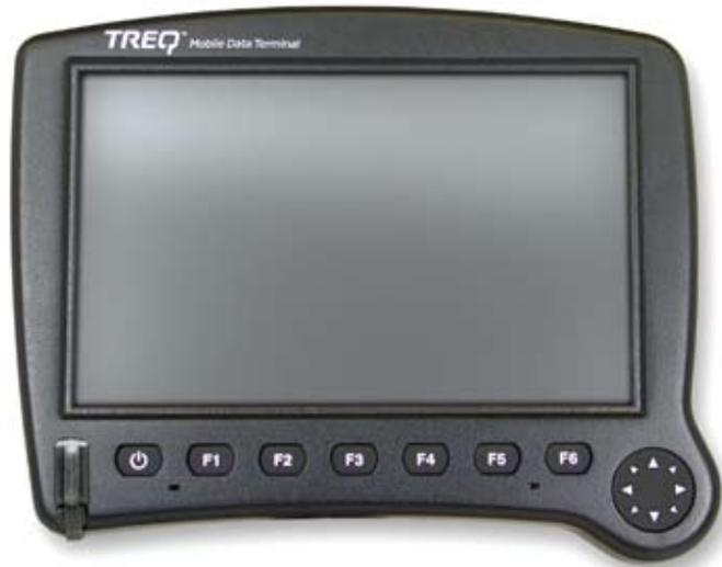
QSI Corporation's TREQ™ is a rugged mobile data terminal intended for use in a wide range of commercial vehicle applications. Patent pending.
