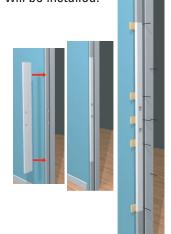
3. Slide Jamb Shield over Jamb. Pre-drill holes into stud and secure piece with screws (included).
