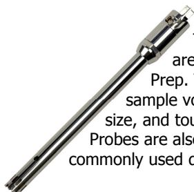
These 10mm Stainless Steel Probes are designed specifically for the Omni Prep. These probes are ideal for larger sample volume, larger initial sample tissue size, and tougher tissue types. Stainless Steel Probes are also resistant to most organic solvents commonly used during homogenization.
