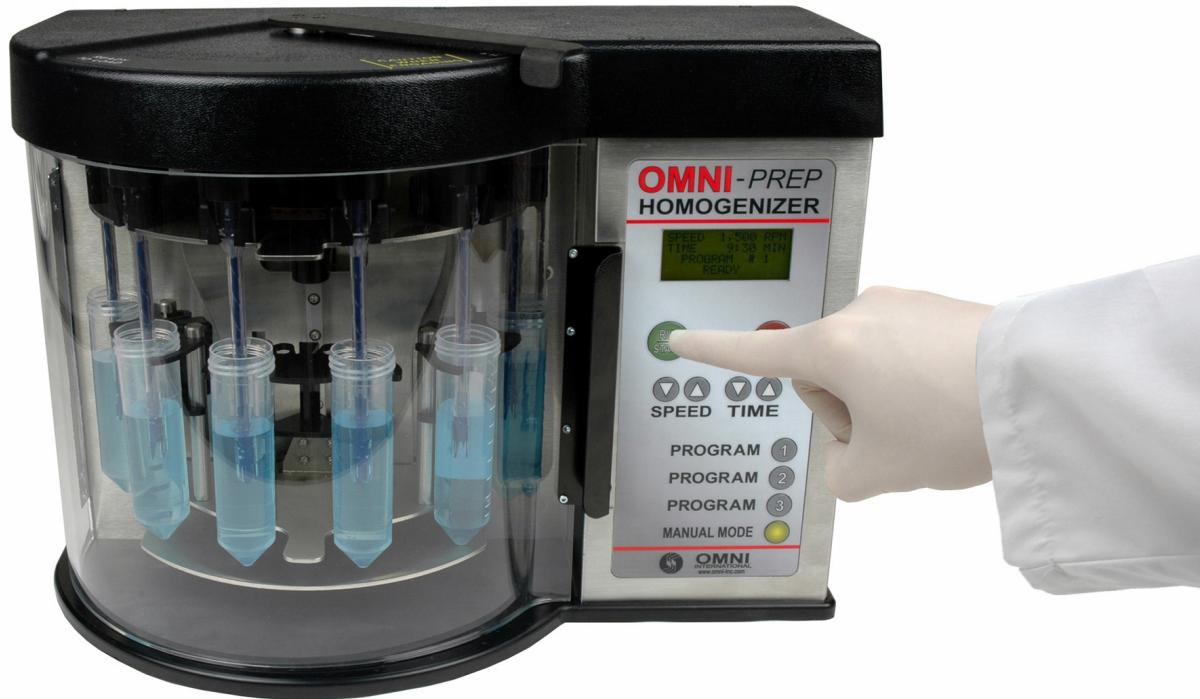
Suitable for processing volumes of 0.25mL to 30mL, the Omni Prep sample racks come in standard tube size configurations and are also available as a custom order for special requirements. Microprocessor control allows the user to program the time and speed of the cycle and free up valuable research time. The Omni Prep is ideal for Pharmaceutical research, Molecular Biology, tissue processing and food and plant analysis.
