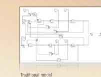
The MapleSim model maps directly to the physical components of the model, whereas the traditional block diagram is much more complex, harder to produce, and looks nothing like the original system representation.
