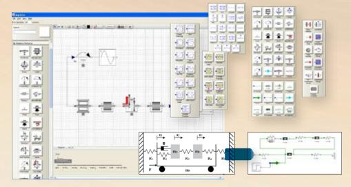
Multi-domain models are easily assembled from pre-built components. MapleSim ships with over 500 components from over 10 domains, including continuous and discrete signals, rotational, translational and multibody mechanics, hydraulics, thermodynamics, and electric circuits. MapleSim recognizes how components can be connected and prevents illogical connections.
