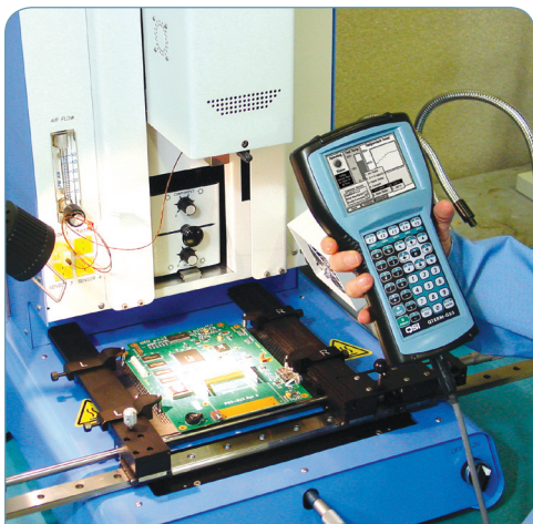
The QTERM-G55 provides control and feedback for a PCB rework station.
