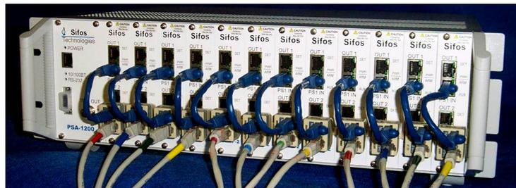
Figure 13: PSA with Port Combiners for High-Power PSE Testing.
