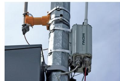
**Licensed 4.9 GHz, Unlicensed 2.4 GHz and 5. GHz:** The MCNU dual radio platform provides simultaneous communications in licensed and unlicensed frequency bands offering wireless broadband access to VII, Public Safety, Public Works and Public Access applications.
