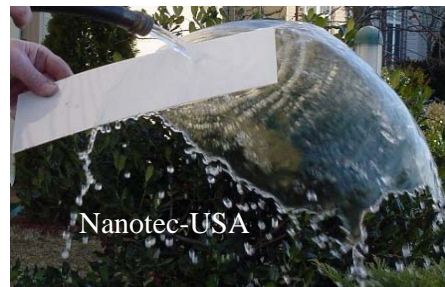
Acry Glo® Aerospace painted panel treated with AeroGuard Paint treatment shows Laminar flow function
