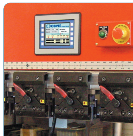
The QTERM-G70 provides valuable information to the user of this metal forming machine.
