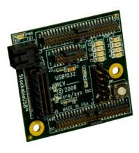
The USB1032 is the ideal module for applications requiring more performance than typical micro-controllers have offered but not needing the full blast offered by an SBC. Wellsuited for applications confined to small, tight spaces, the 125 DMIPS performance requires only 100mA power, considerably less than an SBC.
