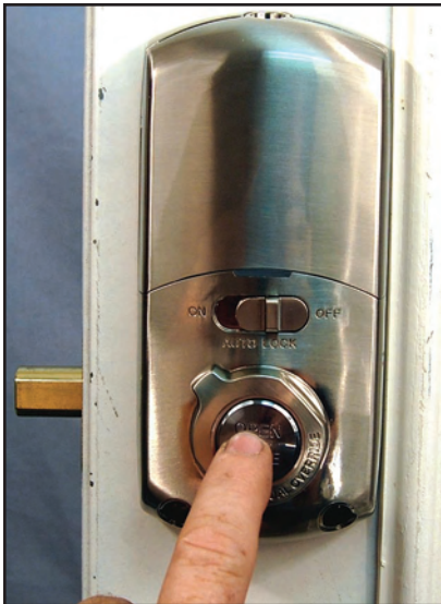
25. Pressing the open/close button will extend or retract the throwbolt.
