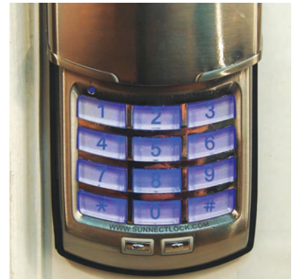
21. Raising the keypad cover activates the keypad and illuminates the keys.
