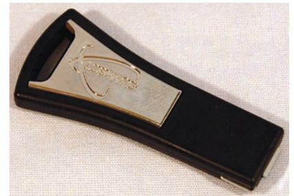
22. The tag keys work on the same principal as an iButton.
