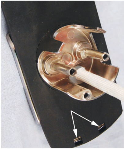
8. Although waterproof, the AP501 is designed with weep holes to allow condensation to escape.
