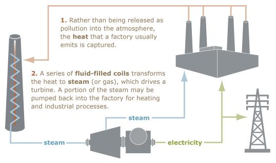
**3.** Steam from the heat recovery boiler is pumped into a **turbine** which generates electricity used to power the plant. Excess power may be sent to the local grid to provide clean electricity for the outlying community.
