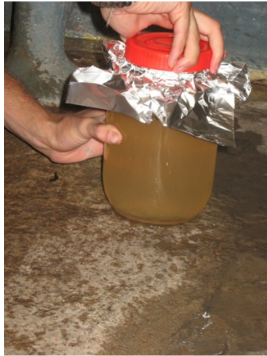
Figure 57: Muddy water from one of the hand pumps
