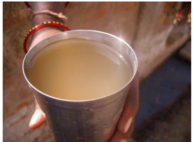
Figure 45: Muddy, yellowish water with bad smell from hand pump H/P ShB 47 in Shiv Nagar. The water cannot be used for drinking.
