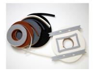
**Closed Cell Silicone Sponge** is heat cured from gum base silicone into molded sheets or rotocured into continuous rolls. High Quality silicone sponge is typically post-cured to improve mechanical properties and high temperature performance. Silicone sponge has a characteristic fabric impression on the skin surfaces. Silicone Sponge generally has better tear and tensile strength than cast silicone foams, making molded sponge a better choice for demanding mechanical applications.
