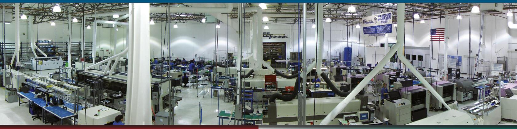
**SMT Services:** 2 Philips/Assembleon SMT lines specializing in odd shapes and prototypes • 2 Philips/Assembleon SMT lines specializing in general production in Reno • 2 Philips/Assembleon SMT lines specializing in general production in Empalme • 1 Prototype and Backup SMT line in Reno • Powerful reflow profiling software and techniques
