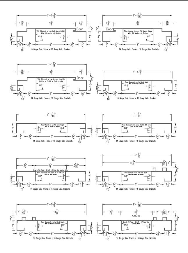
These details are a sample of the different types of frame segments. All NoricF4 frames will be customized to individual building specifications
