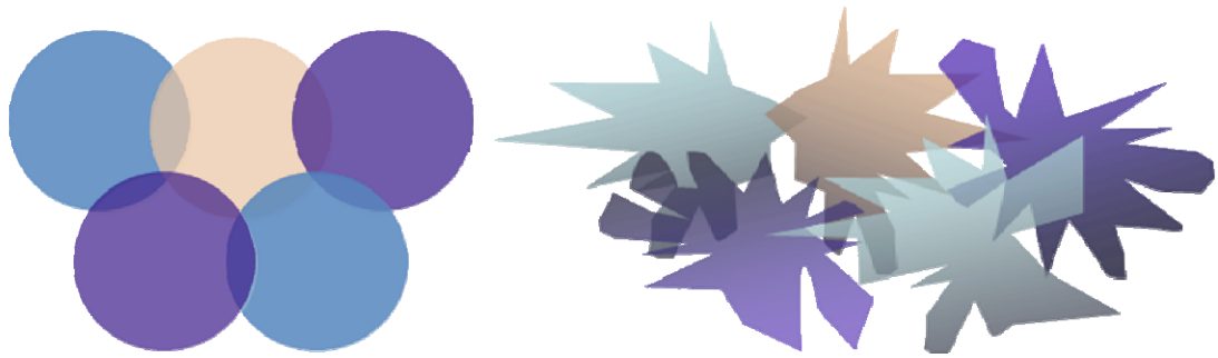
Figure 9: Cell Planning with 3 Non-Overlapping Channels—802.11b/g vs. 802.11n
