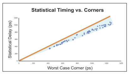
the corner based timing. As this sample of path delays shows, corner based analysis is significantly more pessimistic than the true manufacturing distribution.
