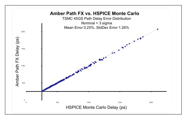
The above figure compares the accuracy of Amber Path FX with SPICE using TSMC 45nm libraries. Several hundred complex test paths (as measured by fanout, depth and cell complexity) are shown here. The path includes data, launch clock and capture clock. This figure compares nominal plus 3 sigma. Over 98% of the paths are within 2% of nominal and nominal plus 3 sigma.
