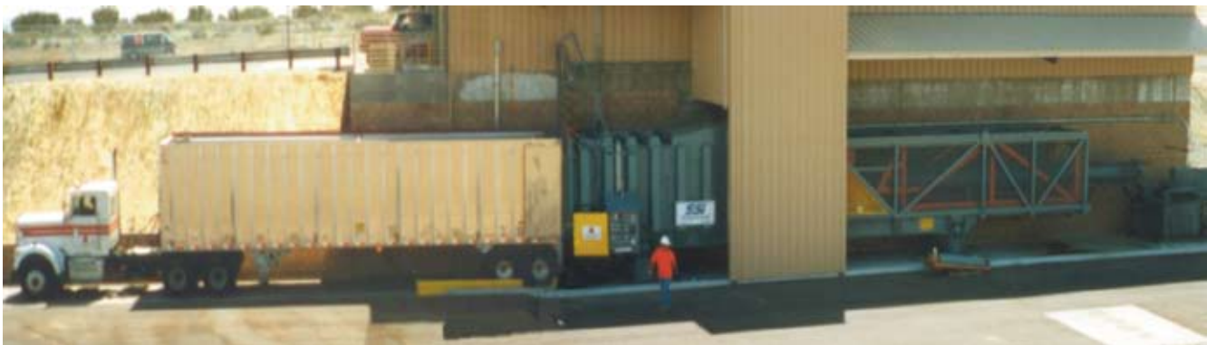
SSI compactors position and balance the legal load while minimizing impact and wear on transfer vehicles.
