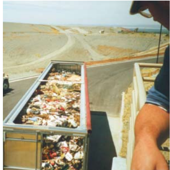
Constant density 25-ton payload in trailer (Top cover removed for photo.)
