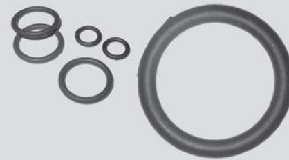
Object: O-ring gaskets. Excess material ("flash") detected at 11 o'clock position.
