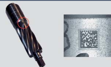
Object: Gear shaft. Data Matrix on gear shaft.
