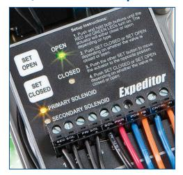
Calibration may be performed quickly and easily using the AXIOM Expeditor's readily accessible membrane control pad. By simply following the on-board instructions, with the unit powered up, all set-up procedures may be performed in a few easy steps and the actuator evaluated for proper stroke timing.
