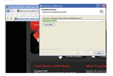
In this example, the end-user is lured to click on a fake Antivirus tool, which actually implants malware into the PC. Even though the user has local admin rights, the installation is blocked. The descendent processes (Total Secure2009[1].exe) of the AppGuard Technology protected IE7 process is also dynamically added to AppGuard Technology protection.
