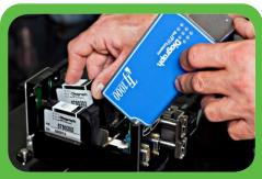
To change ink, just open the hinged cover, snap out the old cartridge, and snap in a new one
