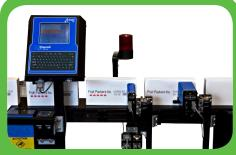
Low-cost, reliable thermal systems offer print speeds up to 200 feet/minute at 300 dpi resolution
