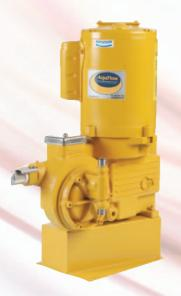
Series 1000 is a rugged, compact, hydraulically actuated and balanced diaphragm metering pump. The pump is available in simplex or duplex configuration, with independent capacity adjustment for each pump head. All drive parts are fully enclosed and operate in an oil bath which minimizes friction and wear while providing protection from harsh environments. A self-compensating hydraulic system assures diaphragm position and eliminates the need for troublesome vacuum breakers and refill valve.
