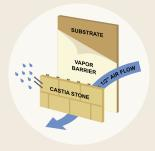
continuous <sup>1</sup>/<sub>2</sub>" gap between the siding and the actual structure. This air space prevents trapped moisture, which can lead to dry rot and mold.
