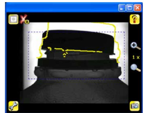
Tilted /Cocked Cap Defect
