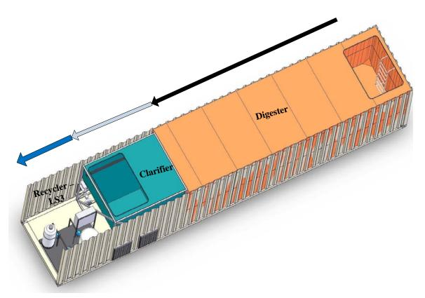
GPD GLOBAL Wastewater-Recycling System - 40' Container 12,000 to 25,000 GPD
