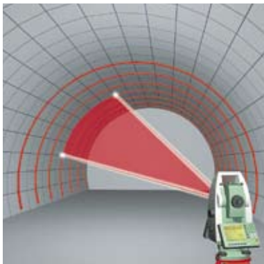
Automatic visualisation of profile anomalies with the VISU function
