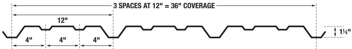
Our 26 gauge Purlin Bearing Rib Panels are far stronger than the commonly used "R" roof panels because they have an extended overlap to provide a leak proof seal. PBR roof panels come standard on all Olympia steel buildings.
