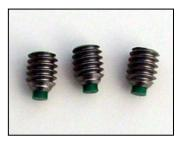
Set screws are used to lock the standard and right angle t-nuts into position. The standard t-nuts included two threaded holes. This allows a set screw to be used in addition to a component like a standoff. Then the component may be removed for a different setup, and the t-nut will remain locked in position. This is very useful for quick change-over where a fixture is used frequently for the same few setups. Be careful not to over-tighten the screws. It is possible to mushroom out the tips.
