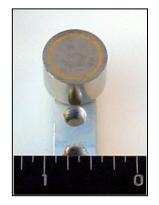
The magnetic locator is  $\frac{3}{4}$ " diameter x  $\frac{1}{2}$ " tall with a flat ground face and nickel-plated case. It has a threaded post that allows it to be attached in many orientations to T-nuts, standoffs, and other locating components.
