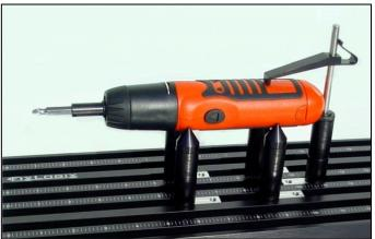
Conical locators are useful for locating in part holes, and for creating simulated Vees. They are available in both 1" diameter and  $\frac{3}{4}$ " diameter sizes. The standard kit includes the larger size, while the small CMM kit includes the smaller. The conicals can be mounted in a variety of positions as shown, and may also be used mounted directly to the swivel head.
