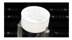
Small pin-standoffs are useful for small parts like soft drink bottle closures. Stainless steel, 2" length x .250" diameter large OD.
