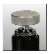
The Mini jackstand detail is a stainless steel platform that is used with a locknut to lock it place once the desired position is set. It may be used on a standoff, or other tooling components with a threaded hole. It may also be used as a clamping device in some setups.
