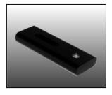
Slide bases are included in the English version kits. The slide base has a threaded hole and a slot. They provide infinite adjustment, allowing components to be set between t-slots. To attach and lock a slide bar, use a locknut and a thumbscrew together through the slot. Use a t-nut in the t-slot and screw the thumbscrew w/locknut into the t-nut.
