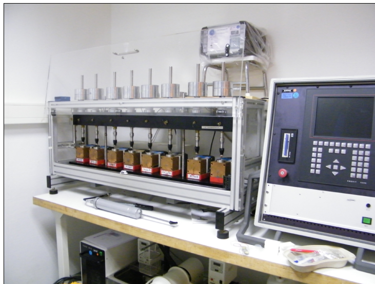
Fig. 2: Assembled test devices in the chewing simulator .
