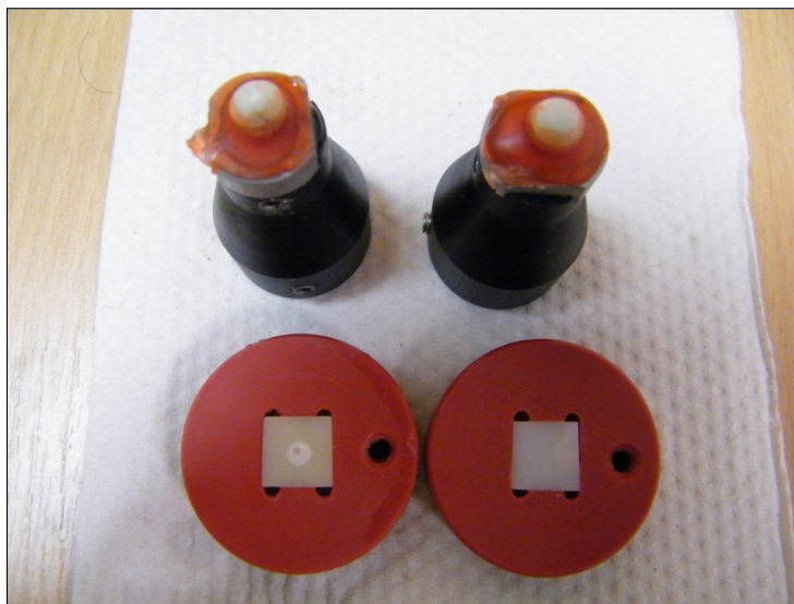
Fig. 3: Embedded Steatite balls in the antagonist holder (top), and samples after finishing the wear test (left: Ceramco®3, right: BruxZir; sample No. 10 each).
