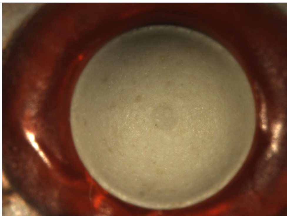
Fig. 7: Situation of the antagonist after the wear test in contact with BruxZir (sample No. 4).
