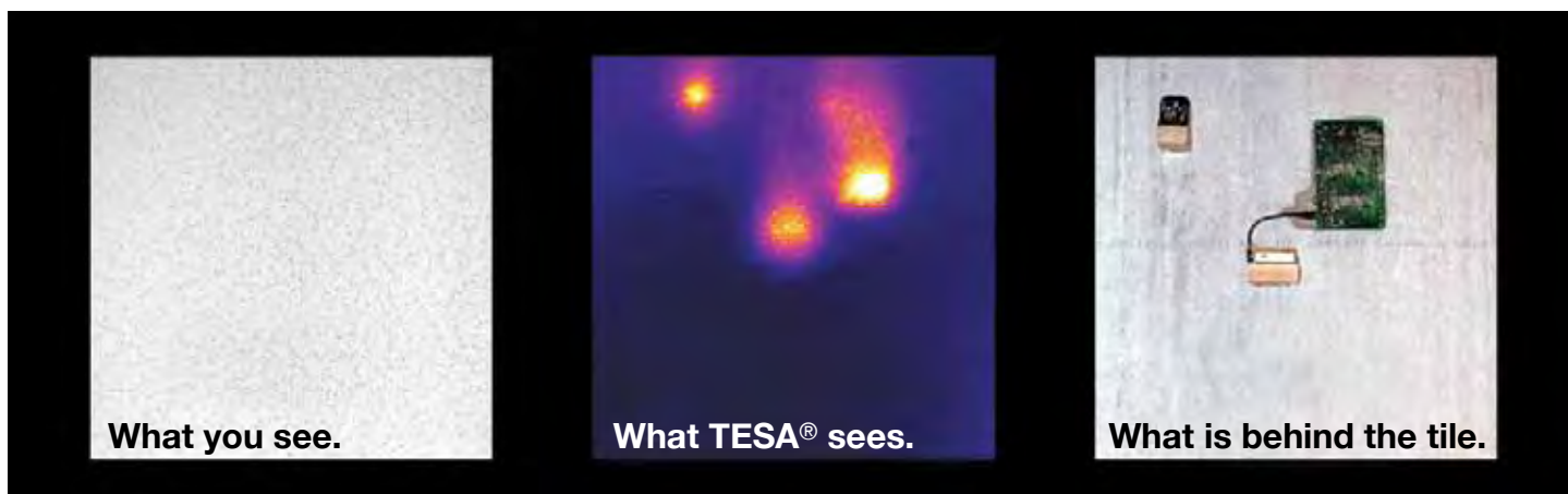
Figure 1. Thermal Emissions Spectrum Analysis ® (TESA) reveals two spycams and a battery hidden behind a ceiling tile. (Source: Murray Associates)
