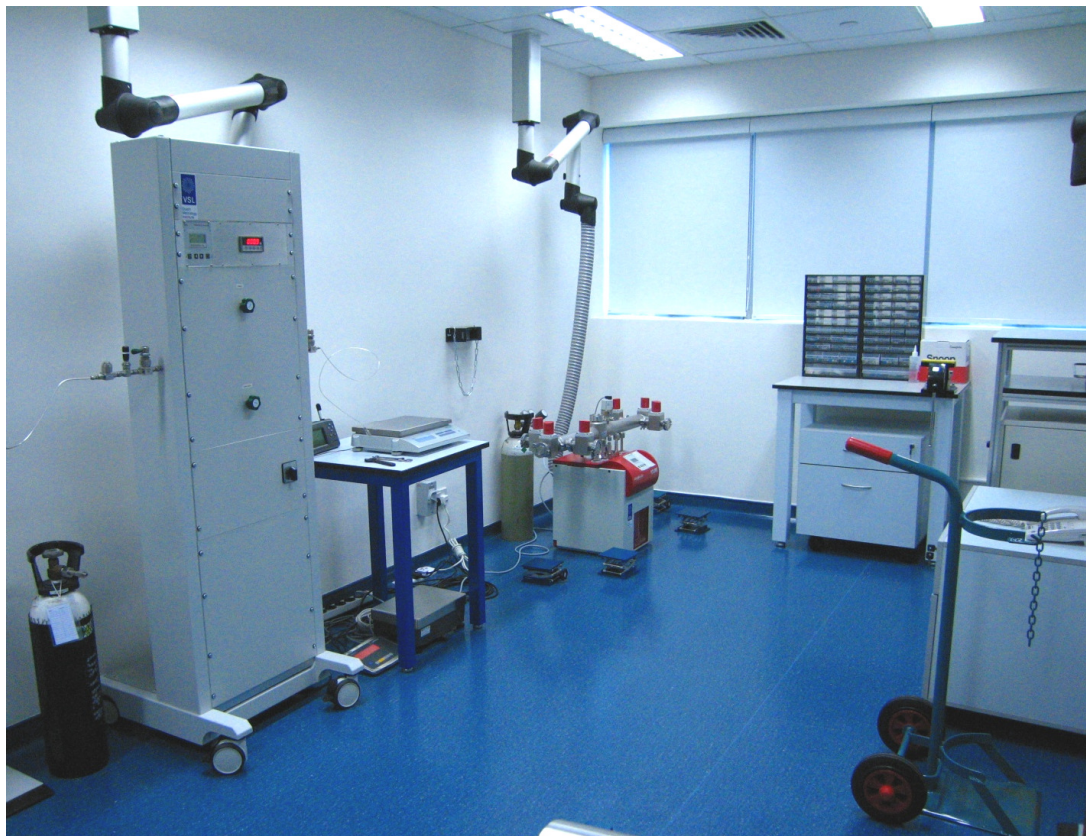
Filling of gas standards using precision gas filling station
