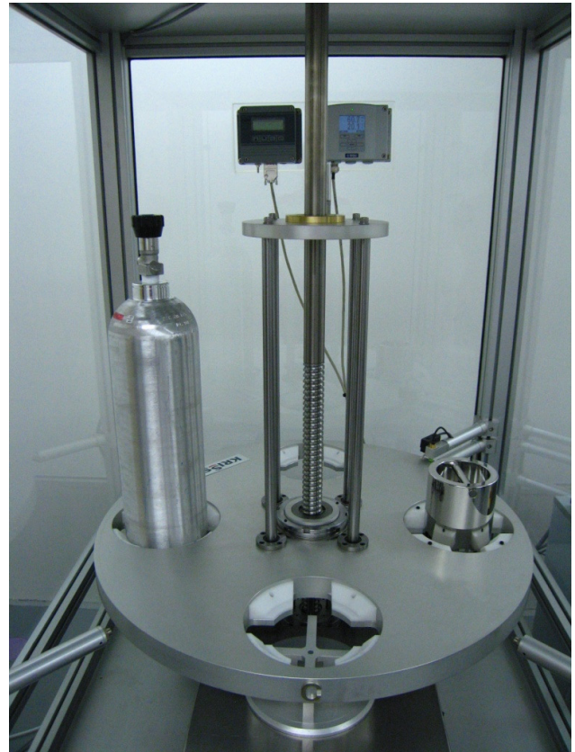
Primary gravimetric system for accurate weighing of gas standards
